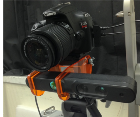
Fig. 1. A Canon Rebel T3 RGB camera and PrimeSense Carmine 1.08 RGB-D sensor pair mounted together.
