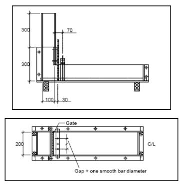
Figure 10 Dimensions and typical design of L-box
