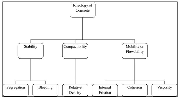
Figure 3 Parameters defining the rheology of fresh concrete.
