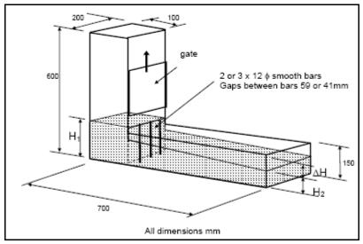
Figure 9 General assembly of L-box
