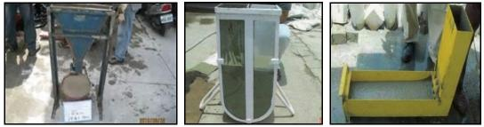
Photograph 2. Test equipments: V-funnel, U-tube, L-box
