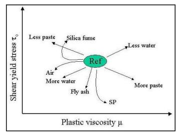
Figure 4 Effect of air, water and additives on rheological parameters
