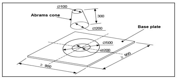
Figure no.7 Base plate and Abram's cone for slump testing
