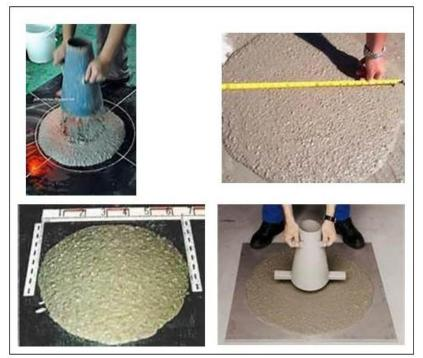
Photograph 3. Slump-flow test
