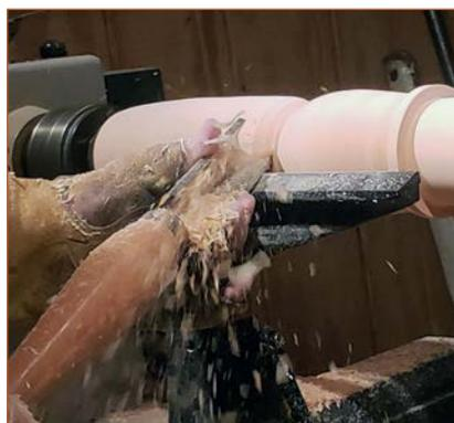
**7. Detailing.** Wing of roughing gouge cuts the quirk between body and head.
