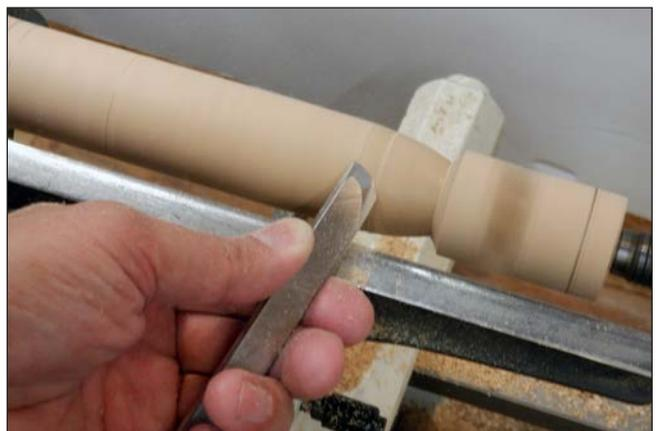
**9. Turning the handle** — Skew chisel pares the curved shapes.
