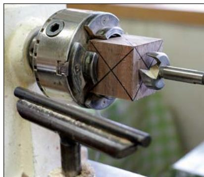
**2. Mount the blank** – in a scroll chuck with side grain facing the tailstock. Use a 1-3/8" (35mm) Forstner bit to bore about 1-1/4" (32mm) deep.
