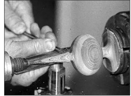
**5. Turn the finial** after regluing the half-balls back together.
