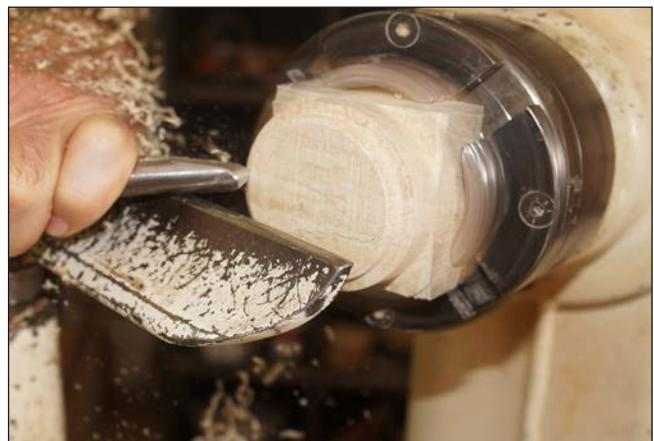
**2. Create a tenon** — Start with the roof, creating a tenon to fit the chuck jaws on what will be the top of the roof.
