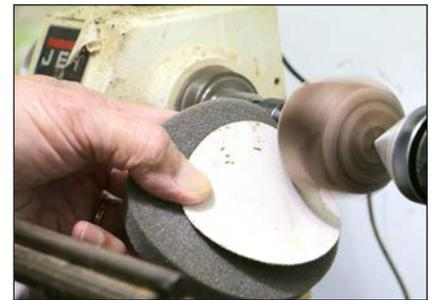
**9. Sand** — *Start with 100 grit and move through 400 grit. A foam pad backing the abrasive will save your fingers and sand the corners evenly.*
