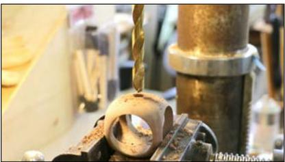
**10. Bore holes** — *Drill a 3/8" hole on the top and bottom of the cube for the finials. With little for a chuck to grip, this is a good operation for the drill press.*
