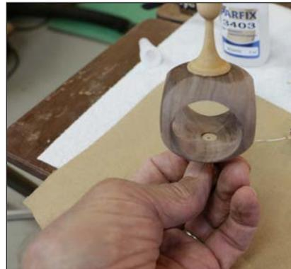
**24. Assemble** – Complete the birdcage and finials, applying finishes and any buffing before gluing in the perch.
