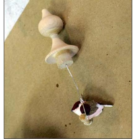
**22. Drill the tenon** – to receive the wire holding the perch.
