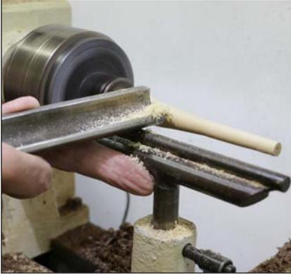
**12. Taper the spindle—** Mount a  $\frac{3}{4}$ "-square x 6" (2cmx15cm) blank in a spigot chuck and taper it toward the tailstock with a spindle roughing gouge.
