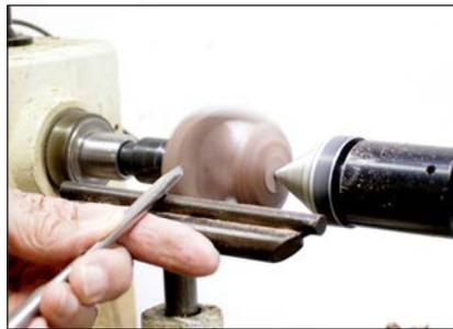
**8. Cut downhill** — *Continue shaping the right and left sides to round the cube. Remember to cut from the largest-to-smallest diameter, cutting downhill toward the tailstock or cup drive.*
