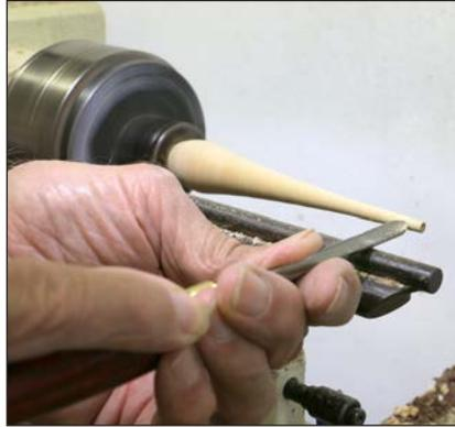
**13. Shape the tip —** Shape with a small spindle gouge or skew. An underhand grip and light touch minimize vibration.
