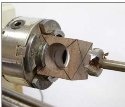
**3. Drill the sides** – Bore holes in all four side-grain sides.
