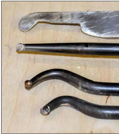
**5. Hollowing tools** — A simple steel scraper, top, can handle the hollowing. I like the new carbide-cup tools. After boring the starter hole, use the straight tool to open it up and make room for the bent tools.
