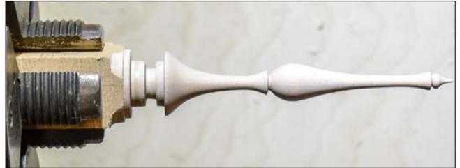
**13. Tenon** — *Measure the hole in the ball and turn a small plug tenon before parting off. There's enough wood left in the chuck for the top finial.*
