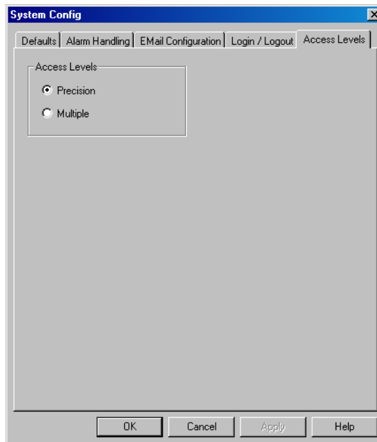
Figure 5-34 System Config-Access levels tab
