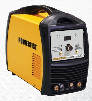
This process uses welding equipment with a high-frequency generator. The arc is created between a non-consumable tungsten electrode and the workpiece. Filler metal may or may not be used, and argon inert gas or intert gas mixtures are used for shielding.
