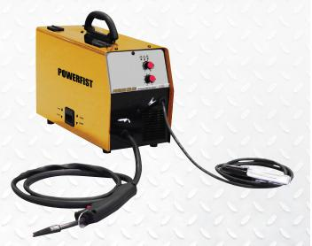
A process that uses a wire-fed welding machine. Metals are melted and joined by heating them with an arc between a continuous, consumable electrode wire and the workpiece. The weld is tubular with flux material contained inside the shielding. Added shielding may or may not be supplied from external gas or gas mixture, depending on the type of flux-cored wire being used.
