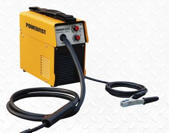
A process used with a wire-fed welding machine. Metals are joined by heating them with an arc, which is between the continuously fed filler metal electrode (solid wire) and the workpiece. Externally supplied gas or gas mixture provide shielding.
