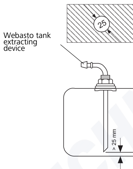
Fig. 804 Webasto tank extracting device (metal fuel tank)
