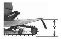
To determine sag, commonly referred to as ride-in, subtract measurement Y from X (Sag=X-Y). Adjust sag by rotating the torsion spring preload cams located on the rear torque arm. See illustration. The ideal amount of sag for this rear suspension is five inches (12.7 cm) (X-Y=5 in./12.7 cm).
