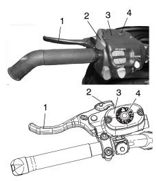
**NOTICE:** If the brake lever is squeezed tightly enough, the lock will move freely into place. Do not force the lock or it may break.
