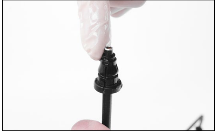
2) Lubricate the inlet hose at the site of the grommet seal.
