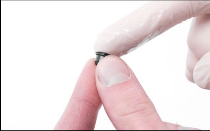
1) Lubricate the new grommet seal with brake fluid.
