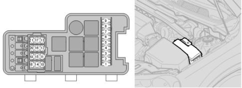
Press in the plastic catches on the short sides of the box and pull the cover upward.
