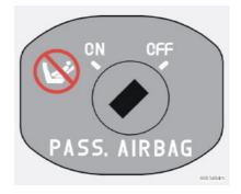
Switch for SRS in ON position.
