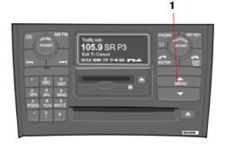
By holding the or word button depressed you can fast forward or rewind in a song or search for a radio station.
