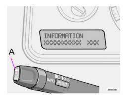
messages stored in the memory by pressing the READ button. Press the READ button to return read messages to the memory.
