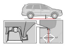
Place the jack under the jacking point and crank it up towards the car floor. Check that the jack sits securely in the anchorage. Then adjust the jack so that its foot is positioned vertically under the anchorage. See illustration. Do not place wood blocks or the like under the jack as you will not achieve full bearing capacity.
