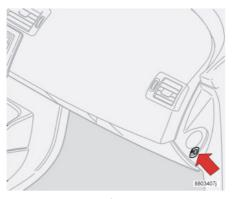
Switch for PACOS (Passenger Airbag Cut Off Switch).
