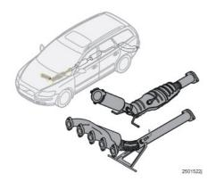
An oxygen sensor monitors the oxygen content of the exhaust gases leaving the engine. This value is fed into an electronic system that continuously controls the injectors. The ratio of air to fuel is continuously adjusted. These adjustments create optimal conditions for efficient combustion, and together with the three-way catalytic converter reduce harmful emissions (hydrocarbons, carbon monoxide and nitrous oxides).
