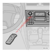
Direct the remote control towards the IR receiver (see illustration) that is located in the dashboard.
