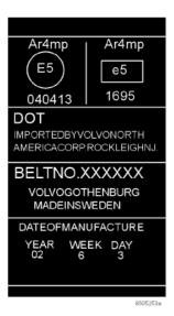
Label on seatbelts with seatbelt tensioner.
