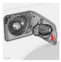
The fuel cap is inside the fuel filler flap on the right-hand rear wing and hangs up on the inside of the fuel filler flap.
