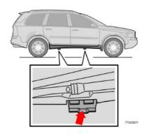
The jacking points are centred under the bottom of the doors.
