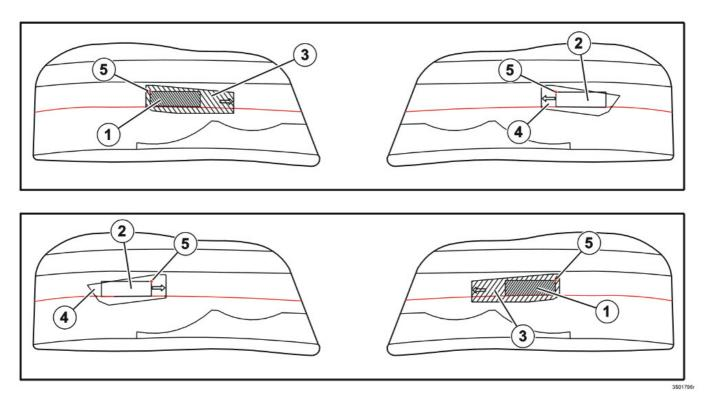
Fitting the mask to the headlamps. The upper illustration is for LHD variants and the lower illustration is for RHD variants. Templates 1 and 2 are for halogen headlamps, 3 and 4 are for Bi-Xenon headlamps.
