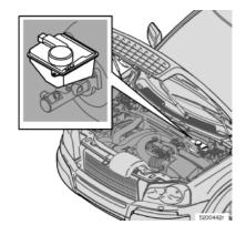
**NOTE!** The fluid should be changed annually for cars driven in conditions requiring hard, frequent braking, such as driving in mountains or tropical climates with high humidity.
