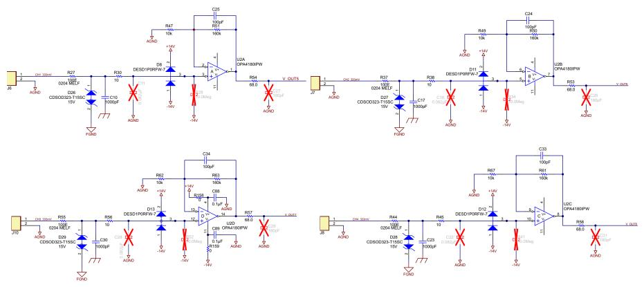
Figure 12. 333-mV Voltage Output Current Sensor Input
