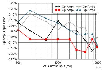
Figure 25. AC Current Input versus Amplifier Output
