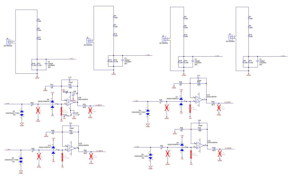
Figure 31. 350-V AC Voltage Input Measurement
