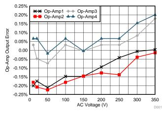
Figure 23. AC Voltage Input versus Amplifier Output
