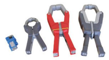
Figure 4. Clamp-On Current Sensors
