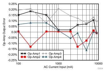
Figure 26. AC Current Input versus Amplifier Output
