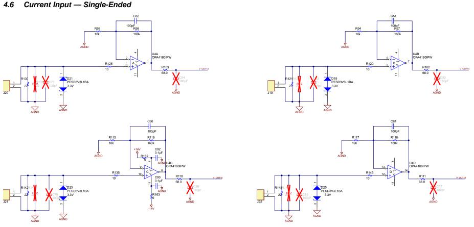
Figure 14. Current Transformer Single-Ended Input
