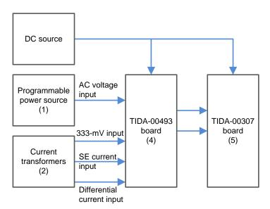
Figure 16. Test Setup for Performance of Measurement AFE
