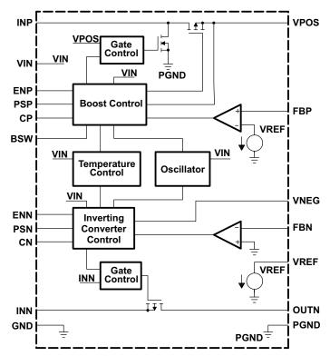
Figure 7. TPS65131 Functional Block Diagram
