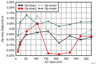
Figure 24. 333-mV Input versus Amplifier Output
