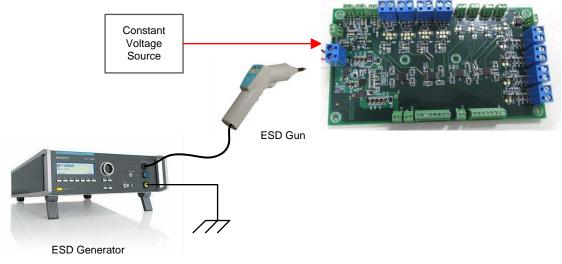
Figure 28. ESD Setup for AFE
