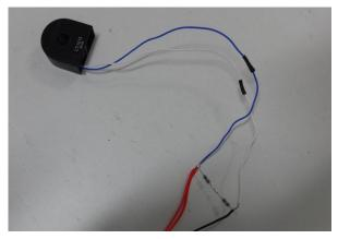
Figure 19. Voltage Output Current Transformer
