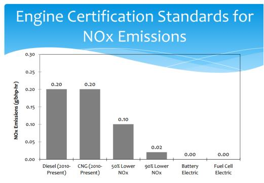
Figure 4 - CARB Engine Certification Standards for NOx Emissions<sup>11</sup>
