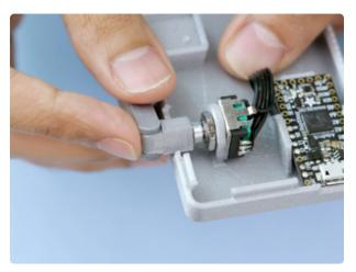
Firmly press the crank onto shaft of the rotary encoder until it's fully seated.
