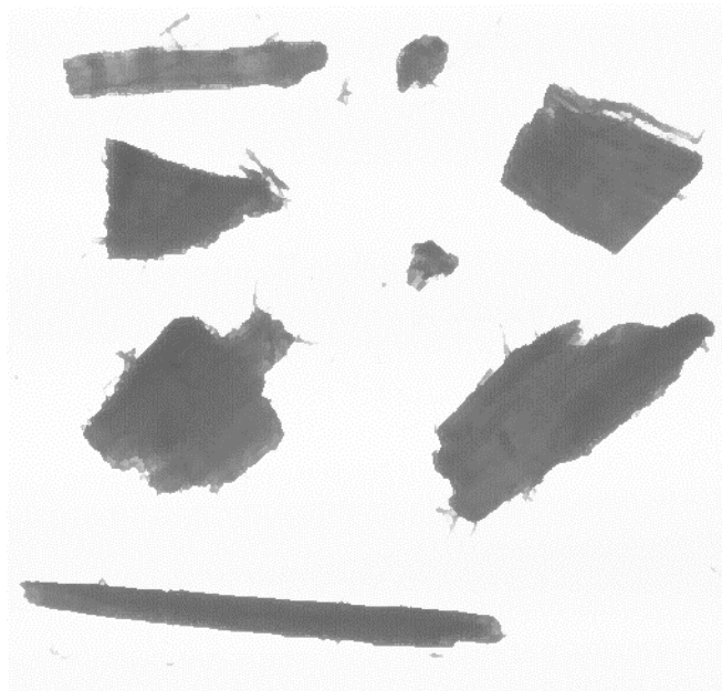
Figure 21. Example of different particle shapes for wood powder.
