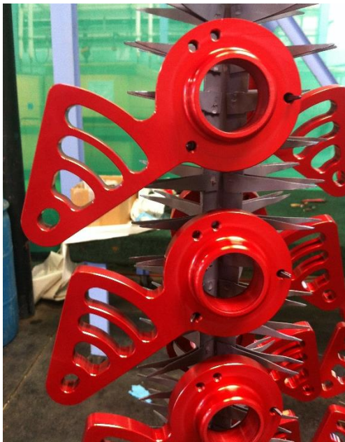
Photo: An example of anodized parts dyed red
