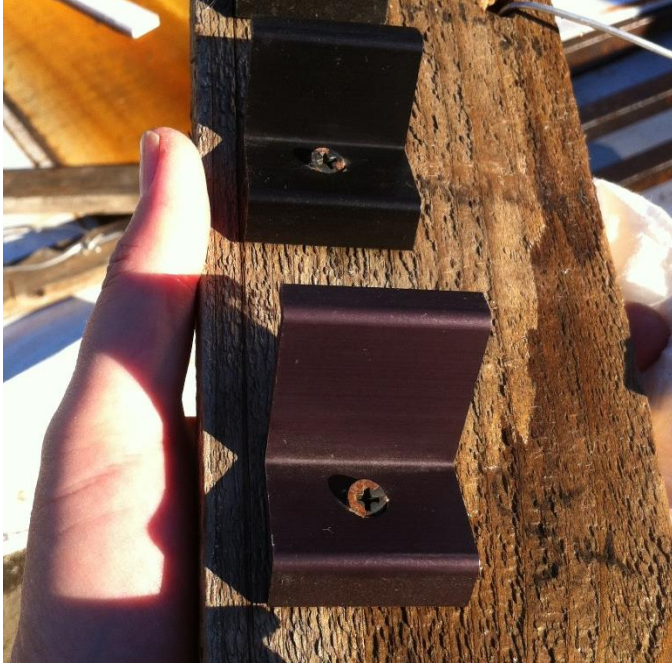
Photo: Two black parts, after being placed in intense direct sunlight for approximately 8 months. Both parts started with a similar black color. The bottom part used common organic black dye and has noticeably faded. The top part was dyed using a 2-step electrolytic process (“architectural anodizing”) and shows no fading.
