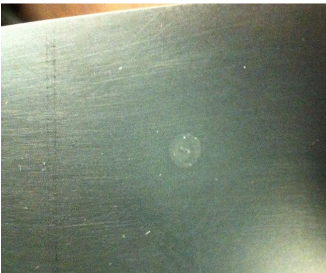
This blemish looks very much like a chemical spot, but it isn't. It's a location where a locating pin inadvertently pushed up the sheet metal. The sheet was peened back into place by the machinist, but the cold work altered the material enough to change the color of the anodizing.
