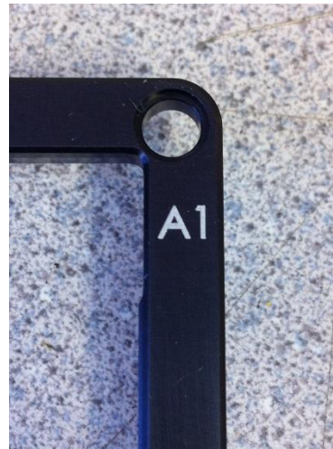
An example of laser engraved characters on a black anodized part.
