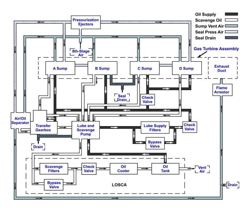
Adapted for testing purposes only from Gas Turbine Systems Technician (Electrical) 3/ Gas Turbine Systems Technician (Mechanical) 3, Volume 2
