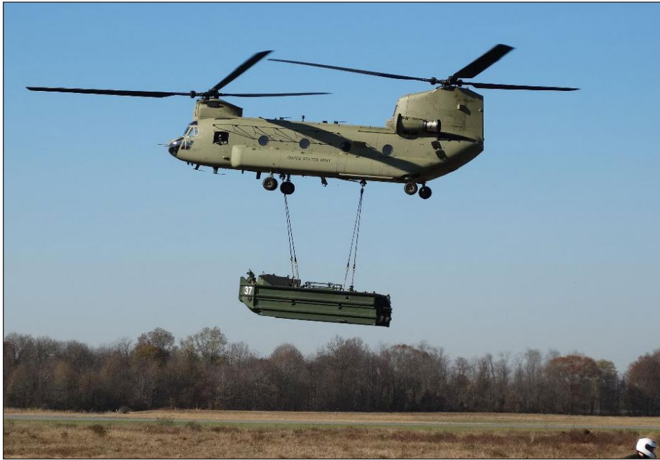
A CH-47 helicopter flies the BEB as a sling load.
