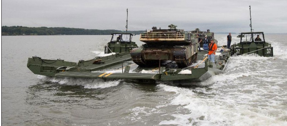
In a military load classification 140 longitudinal rafting test, a Bridge Erection Boat carries two M1A1 Abrams tanks in the C&D Canal.
