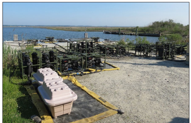
USMC LWPS seawater testing at Wallops Island, Virginia.
