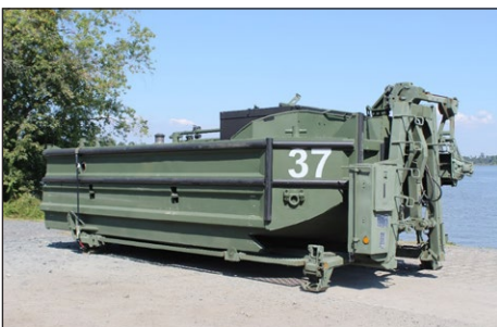
The BEB, loaded on a bridge adapter pallet.
