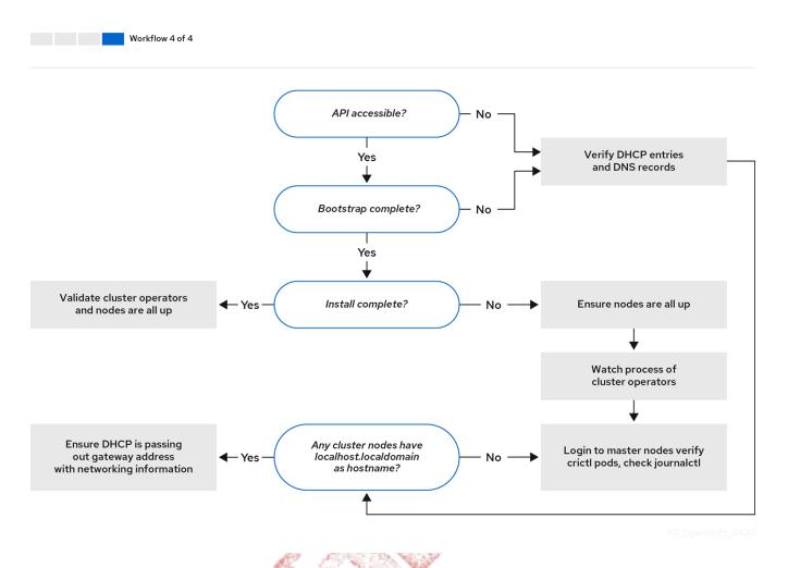
*Workflow 4 of 4* illustrates a troubleshooting workflow from a non-accessible API to a validated installation.
