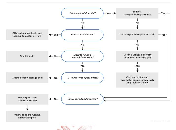
*Workflow 2 of 4* illustrates a troubleshooting workflow for bootstrap VM issues, bootstrap VMs that cannot boot up the cluster nodes, and inspecting logs.
