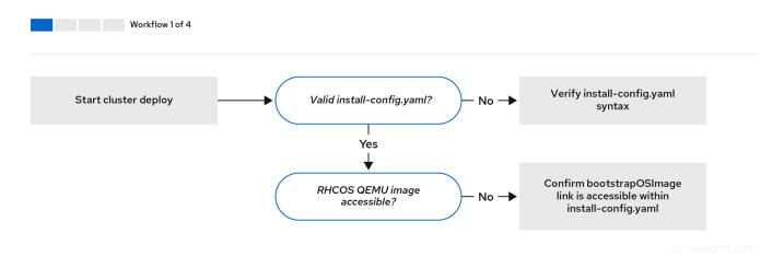
*Workflow 1 of 4* illustrates a troubleshooting workflow when the install-config.yaml file has errors or the Red Hat Enterprise Linux CoreOS (RHCOS) images are inaccessible. Troubleshooting suggestions can be found at
