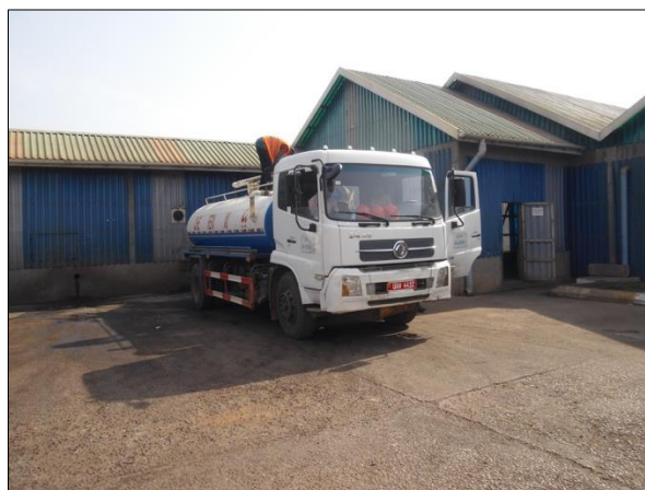
Figure 1. A truck arriving at the treatment plant emptying, faecal sludge from pit latrines and septic tanks.
