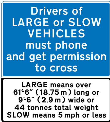
May be used with diagram 786, 787 or 788. "must phone" may be varied to "must use SOS phone"
