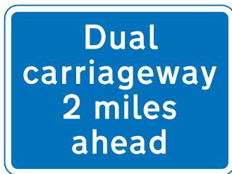
Figure 5-5 Diagram 818.1 (S11-2-11) Section of dual carriageway ahead (distance may be reduced or omitted)
