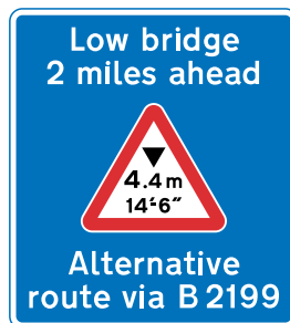
Figure 7-17 Signs on approach to an arch bridge with a diversionary route
