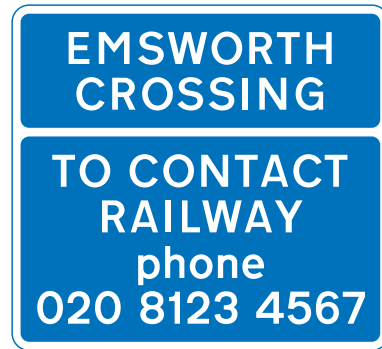
The name of the crossing may be varied and displayed on any number of lines. "TO CONTACT RAILWAY" may be on one line, "RAILWAY" may be varied to "TRAM Co." and the telephone number varied. May be used with diagram 782 or 783
