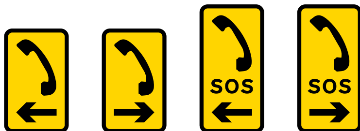
Figure 20-22 Diagram 788 (S11-2-72) Direction to telephone or emergency telephone at or near a railway or tramway level crossing (Alternative types)
