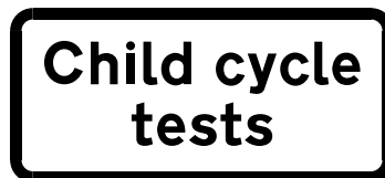
May be used only in combination with diagram 950. “tests” may be varied to “training”. “Child cycle tests” may be varied to “Cycle crossing”, “Cycles crossing” or to “Cycle event”. A distance, an arrow or both may be added
