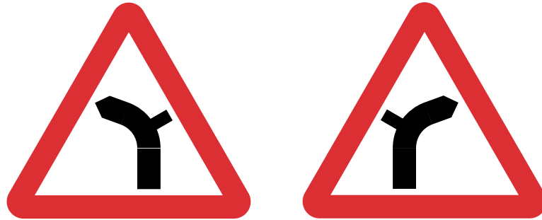
Figure 3-2 Diagram 512.1 (S2-2-9) Junction on the outside of a bend ahead (Alternative types)
