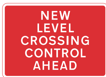
Figure 20-24 Diagram 790 (S14-2-67) New method of controlling traffic at a railway or tramway level crossing ahead
