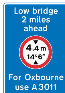
Figure 7-13 Signs on approach to a non-arch bridge with a diversionary route
