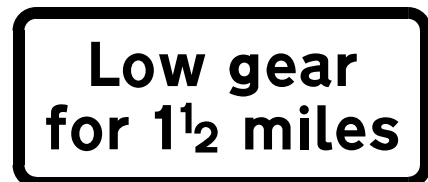
May be used only in combination with diagram 523.1 or 524.1. The distance may be varied.
