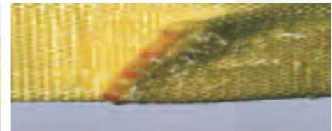
Broken or worn stitching in load bearing sew patterns
