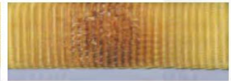
Melting or charring of the tiedown, or weld splatter on the tiedown
