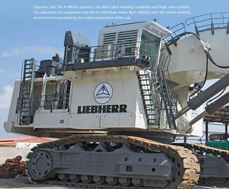
The hanging arch hose arrangement provides direct visibility over large areas of the upper carriage. Additionally, a camera system shows areas that can't be observed directly. The electronic machine controls assure the best operator performance throughout each shift. Furthermore, the ergonomic component access and long service intervals assist the service team to ensure more uptime.
