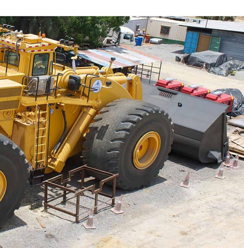
The L-2350 wheel loader, with an operating capacity of 72,574 kg (160,000 lbs.), can center load haulage trucks with payload ratings ranging from 320 to 400+ tons. The most powerful and productive wheel loader in its class, the L-2350 is part of the Generation 1 wheel loader line,
