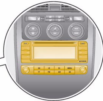
Control unit with display for radio and navigation J503 or Radio R in centre console
