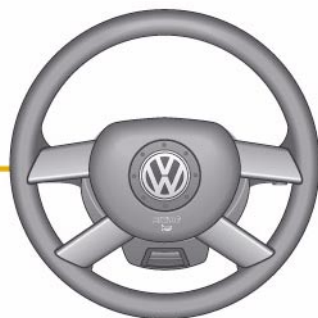
Steering wheel operating unit E221 Slave control unit in LIN data bus
