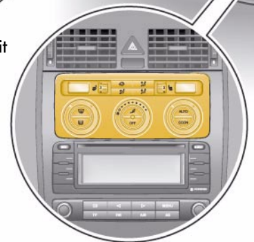
Climatronic control unit J255 in centre console
