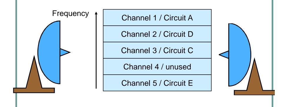
In FDM, each circuit is sent in a separate channel. If channel bandwidth is large, there will be fewer channels. Voice uses 4 kHz channels to allow more channels.
