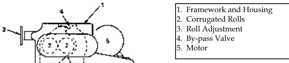
Figure 6 - A Typical Crumbling Roll
