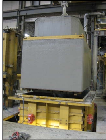
Fig. 34: Dry Cast Box Stripped from Form
