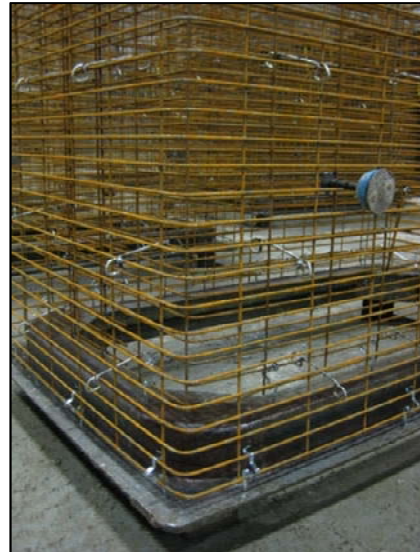
Fig. 24: WWR Cage Assembled on Pallet
