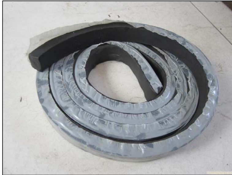
Fig. 42: Butly Mastic Used for Compressible Joint Filler
