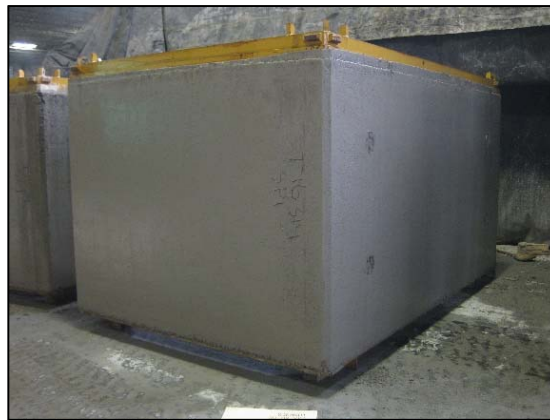
Fig. 35: Dry Cast Box Ready for Curing
