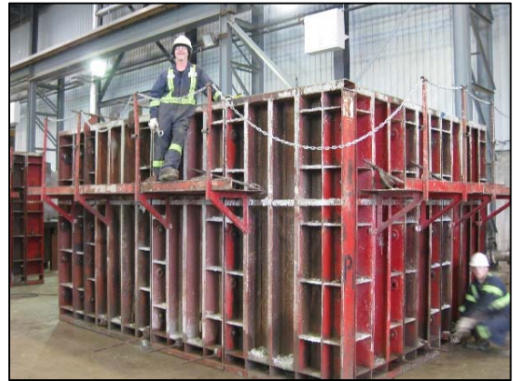
Fig. 31: Wet Cast Form Assembled
