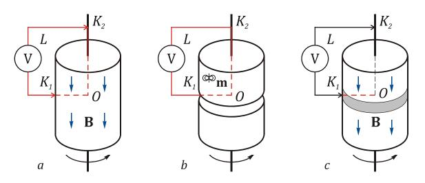
Fig. 5.1. Unipolar generator with a permanent rotating magnet
