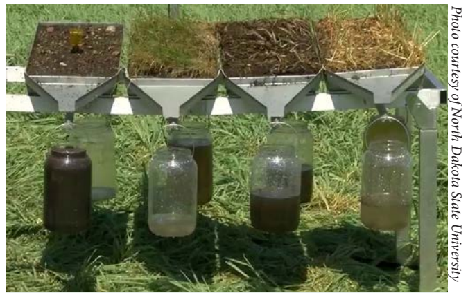
This rainfall simulator shows the effect of healthy and covered soils versus uncovered and unhealthy soils. The runoff water from the simulator is shown in the front row of jars. Trays 1 and 3 (uncovered soils) show significant runoff and sedimentation. The back row of jars shows rainfall infiltration through the soil profile and trays 2 and 4 (covered soils) show significant infiltration.
