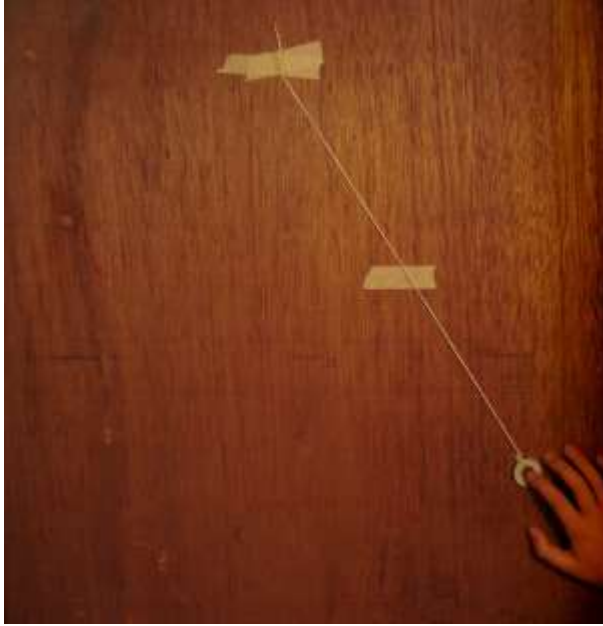
Figure 1: This figure shows the string taped to the wall at the top with a washer attached to the end. The other piece of tape has a red X on it marking the angle at which we will release the pendulum each time. It should be high enough so that it will work for the short, medium, and long pieces of string.
