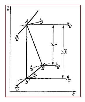
$$\begin{array}{ll} compressio & n & \eta_i = \frac{\Delta t_{ad}}{\Delta t} = \frac{T_D^{'} - T_S}{T_D - T_S} = \frac{\Delta i_{ad}}{\Delta i} = \frac{i_D^{'} - i_S}{i_D - i_S} \\ \\ \exp \ ansion & \eta_i = \frac{\Delta t_{ad}}{\Delta t} = \frac{T_D - T_S}{T_D - T_S^{'}} = \frac{\Delta i_{ad}}{\Delta i} = \frac{i_D - i_S}{i_D - i_S^{'}} \\ \end{array}$$
