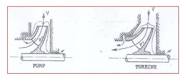
If  $\Delta V$  is the total leakage , the volume flowing through the rotor channels is:
