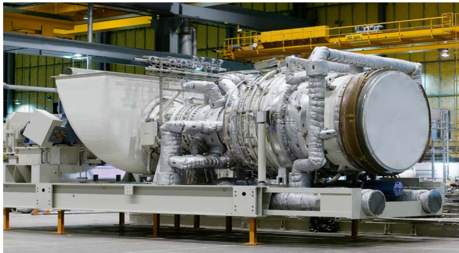
Figure 3(a): The Land-based gas turbine SGT-800 for power production, real life image [5]
