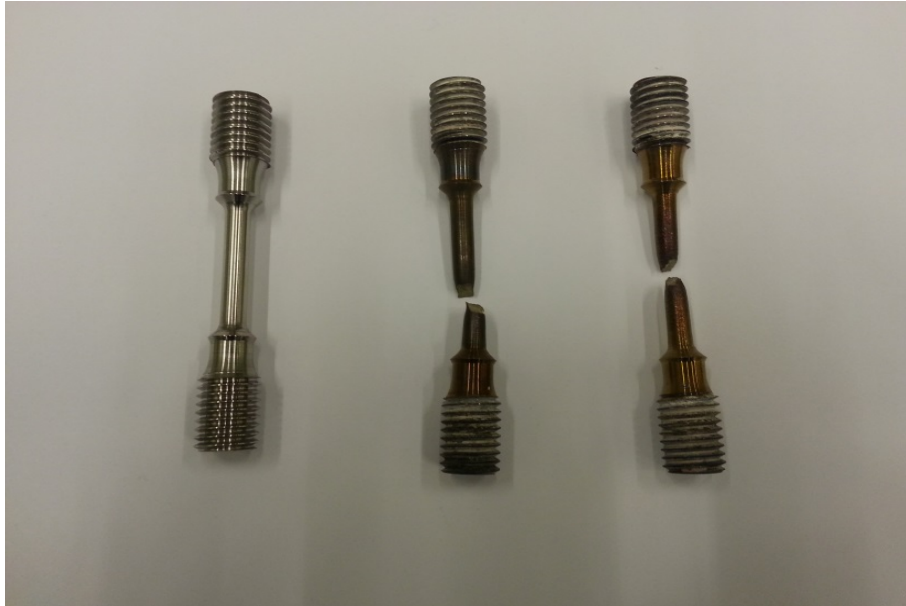
Figure 38: Specimens Of In718 before and after tensile test of specimen A and B shows ductile failure
