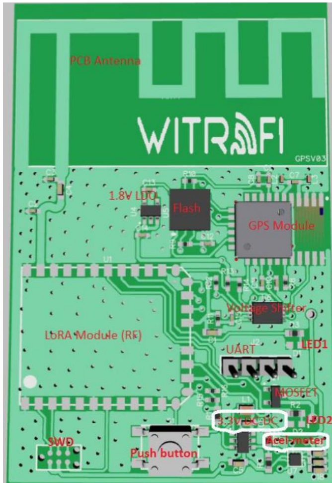
Figure 17: WinNode Board components –final version.
