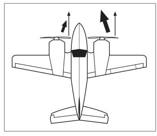
Figure 1-3. Yaw force due to P-factor
