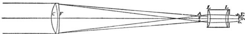
Diagram of a refracting telescope. CF represents the objective lens and LL the eyepiece. The observer's eye is identified by E.
