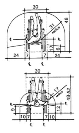
NOTE: Motorized wheelchairs may extend ground space to a length of 52"
