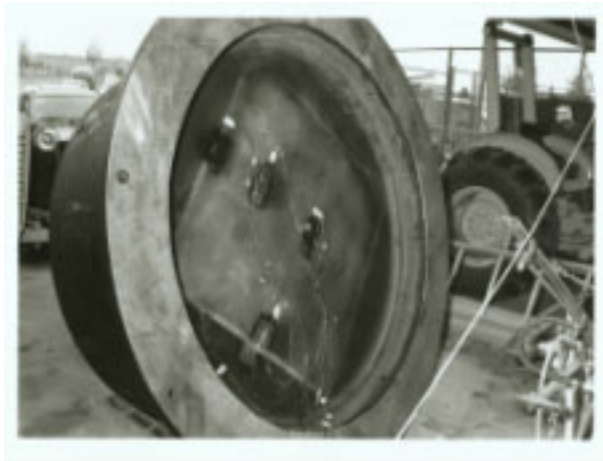
HSLA-100 Holding Bulkhead Panel Model: Before Test (Left) and After Hydrostatic Test to Rupture (Right)
