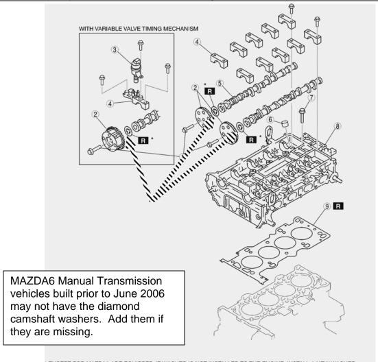
\*: EXCEPT FOR MAZDA6 ARE EQUIPPED. IF WASHER IS NOT INSTALLED TO THE ENGINE, INSTALL A NEW WASHER.
