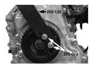
3. Rotate the crankshaft clockwise using the crankshaft pulley bolt until it stops turning (held by the timing peg).
