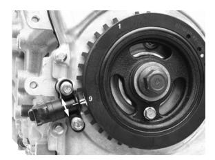
• California specification LF engines: align the CKP sensor with the centerline of the 4<sup>th</sup> tooth down from missing teeth as pictured.
