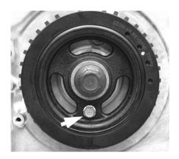
8. Remove the crankshaft timing peg 303-507.
