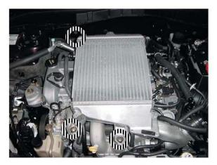
C. Remove the air bypass control hose clamp and disconnect the hose from the valve.
