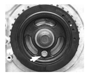
21. Remove the crankshaft timing peg 303-507.
