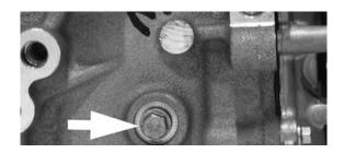
10. Install the cylinder head cover and tighten in sequence to 8.0-11.5 Nm (70.9-101.7 inlbf).
