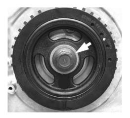
4. Remove the crankshaft pulley bolt.
