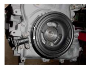
• L3T Engines the correct timing mark is 20 teeth back from the missing tooth.
