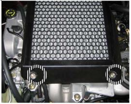
B. Remove the three 12 mm bolts securing the intercooler to the intake.
