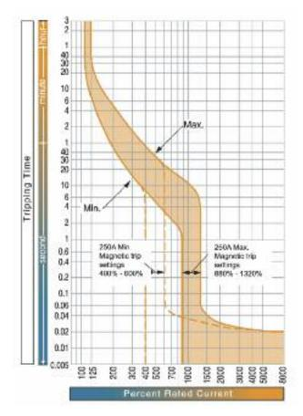
YB3N & YB3S 3 and 4-pole Time/Current Characteristics for 250A
