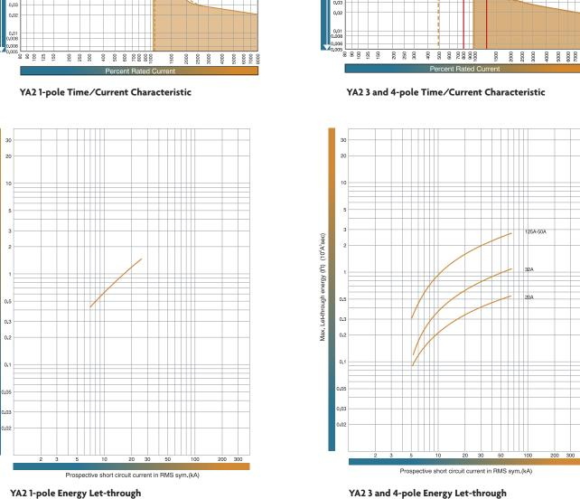
Magnetic trip current  $I_{\rm R}$ (A) 1 50 40 30 (A) 1250 +/- 250 1200±240 756±151 600±120 384±77 125 100 20 63 50 10 8 6 5 4 3 240±48 50' 100A (max) 1 50 40 50' 100A (min) 20`32A(max) 30 20 Tripping Time 10 8 6 5 4 125A (max) 20`32A(min) 3 2 0.8 0.6 0.5 0.4 0.3 0.2 Adjustable setting range of magnetic trip 0.1 0.08 0.06 0.05 0.04 0.03 LO 5000 6000 7000 8000
