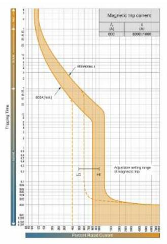
YA6 Time/Current Curve (Thermal / Magnetic 800A)
