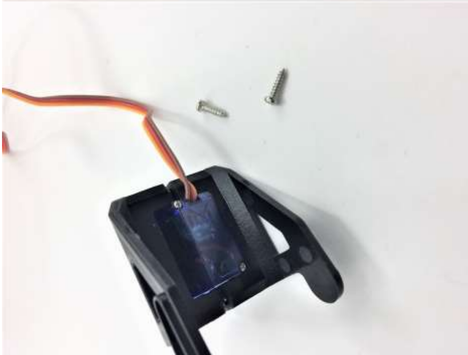
Use two self-tapping screws (in the FPV package) to tighten
