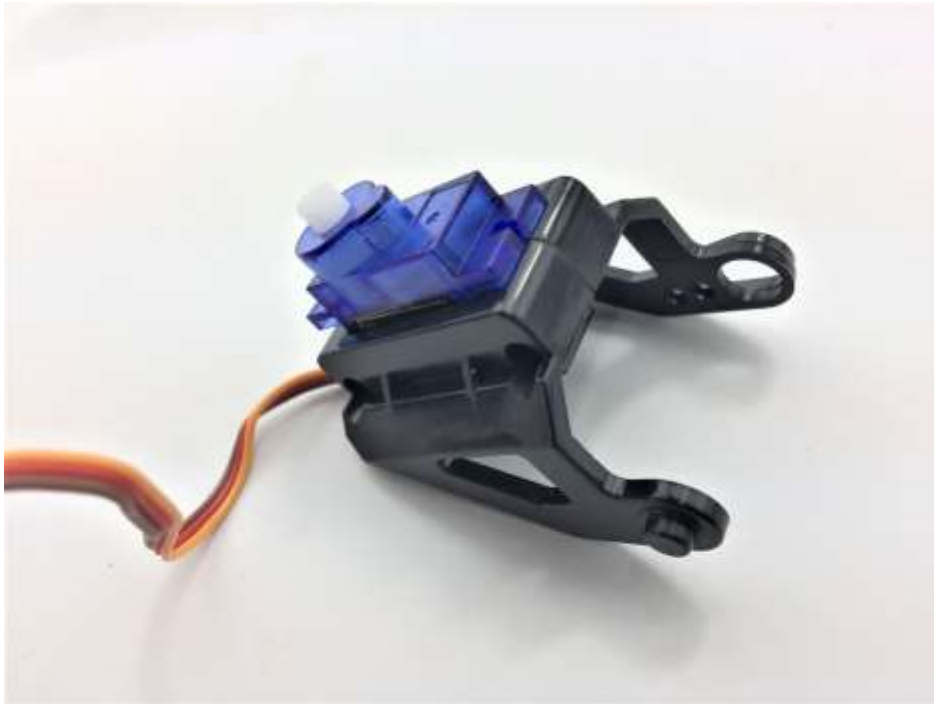
Assemble the FPV holder and servo
