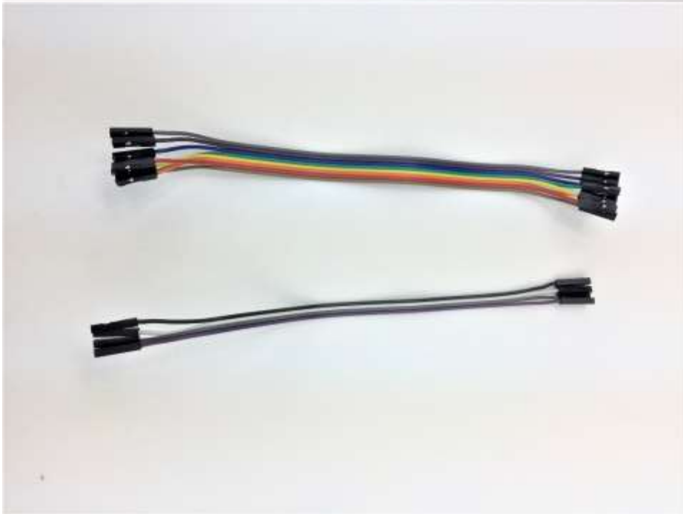
Separate the jumper cable set into four and eight configurations
