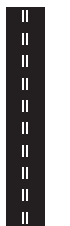
Reversible lane markings (lane which may be used for alternating direction of traffic flow)
