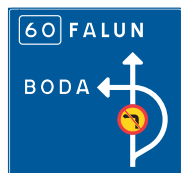
Advance direction sign diagrammatic type indicating prohibition of left turning
