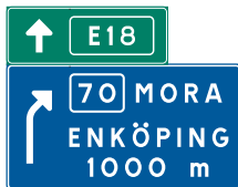
Advance direction sign exit ahead
