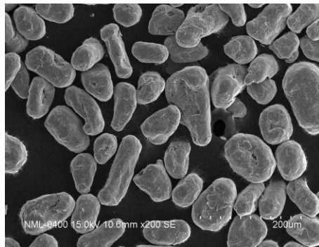
Figure1.- SEM micrograph of annealed low carbon content ferrous powders
