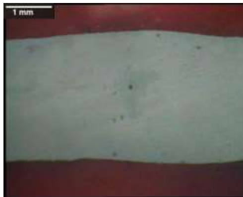
Fig. 13: Optical microscopy image of the welded zone at the cross section of both sided TIG welded Aluminium samples with current setting of 150 A and welding speed(a) 3.5 mm/s (b) 4 mm/s (c) 4.5 mm/s (d) 5 mm/s
