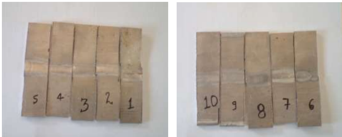
Fig. 4–welded specimen performed with (a) welding speed 3.5 mm/s and welding current 100, 110, 120, 130 and 140 A for sample no 1, 2,3,4,5 respectively (b) welding speed 4 mm/s and welding current 100, 110, 120, 130 and 140 A for sample no 6,7,8,9,10 respectively
