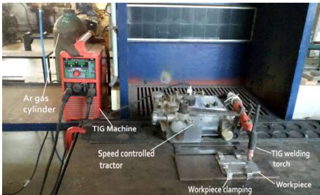
Fig. 3 – Experimental set-up for TIG welding
