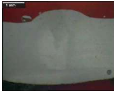
Fig. 13: Optical microscopy image of the welded zone at the cross section of both sided TIG welded Aluminium samples with current setting of 150 A and welding speed(a) 3.5 mm/s (b) 4 mm/s (c) 4.5 mm/s (d) 5 mm/s
