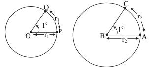
In figure we draw two circles of different radii  $r_1$  and  $r_2$  and centres O and B respectively. Then the angle at the centre of both circles is equal to  $1^c$ . i.e.,  $\angle POQ = 1^c = \angle ABC$ .
