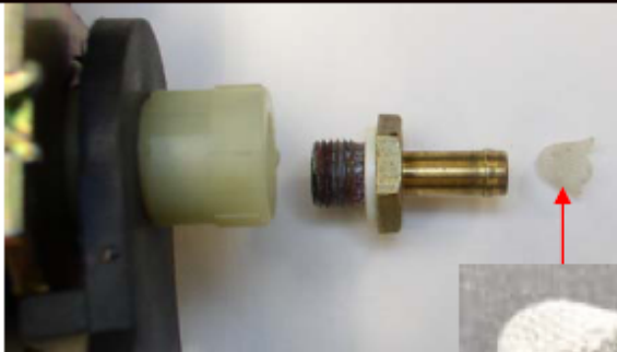
Filter in the inlet fitting prior to Jun '07
