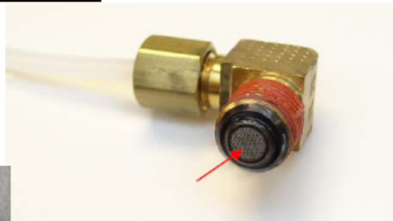
Filter on the outlet fitting prior to Jun '07
