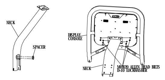
Remove the cover from the power cord access hole in the treadmill neck. If not preassembled, slide the neck shroud onto the treadmill neck.
