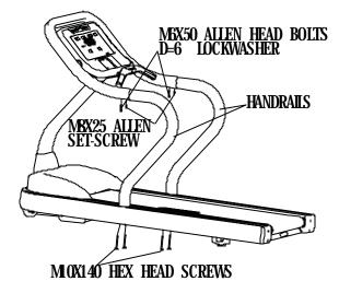
If necessary, rotate the handrail slightly to align the display console handrail stub with the threaded hole in the handrail connecting tube. Secure the handrail to the display console with two M6 X 50 Allen head bolts and D=6 lockwashers two M8 X 25 Allen Set-Screw. Secure the handrail to the treadmill base assembly with two M10 X 140 hex head screws. Tighten all screws securely.
