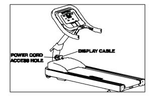
Slide the neck shroud down into position on the base assembly shroud to cover the display cable.
