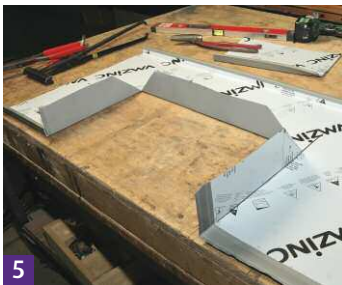
6 Position and then solder corner gussets.
