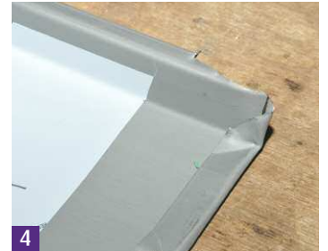
4 Create safety check at top of panel.
