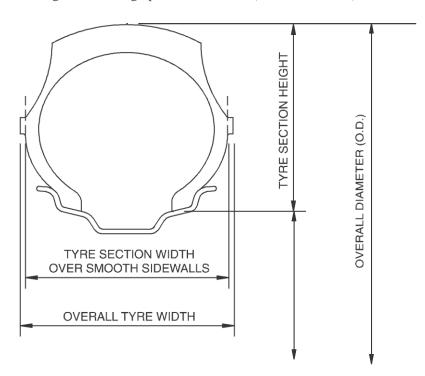
**Tyre Overall Diameter -** This is the diameter of an inflated tyre at the outermost surface of the tread, or twice the inflated Section Height of a tyre, plus the nominal Rim Diameter.
