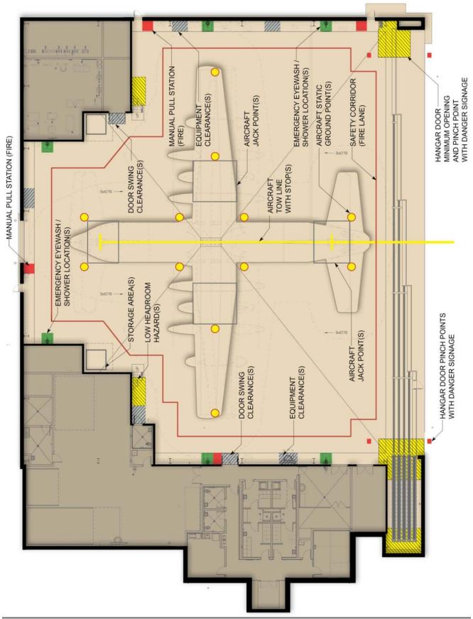
Appendix A: Example Hangar Floor Marking Plan:
