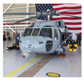
rating. UFC 3-575-01 (Figure 2-3) requires static ground points to be 18-inch diameter yellow circle with a 2-inch wide red border and black text. The pre-decisional version of UFC 4-211-01 will reference UFC 3-575-01 Figure 2-3 for Army, Air Force and Navy hangars when approved and issued.
