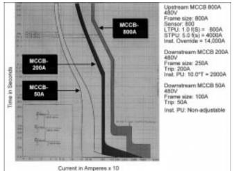
Fig. 4. Time-current curve with upstream 800-A MCCB.
