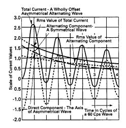
Fig. 1. Structure of an asymmetrical current wave.
