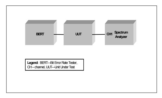
Figure 1.6. Equipment Configuration for Output Power Measurements
