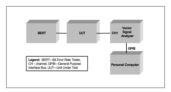
Figure 1.5. Equipment Configuration for Data Analysis
