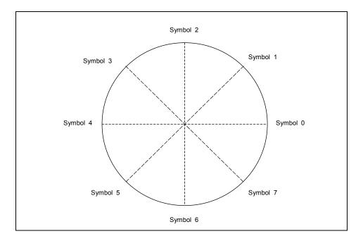
Figure 1.1. Phase State Encoding
