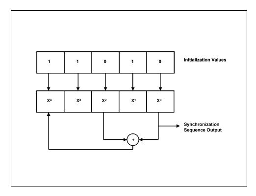
Figure 1.3. Synchronization Sequence Generator
