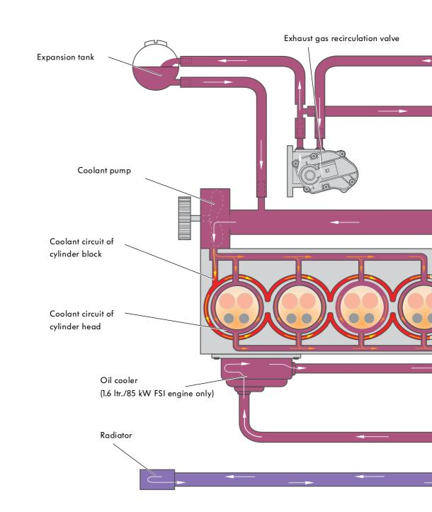
The dual circuit cooling system has the following advantages:
